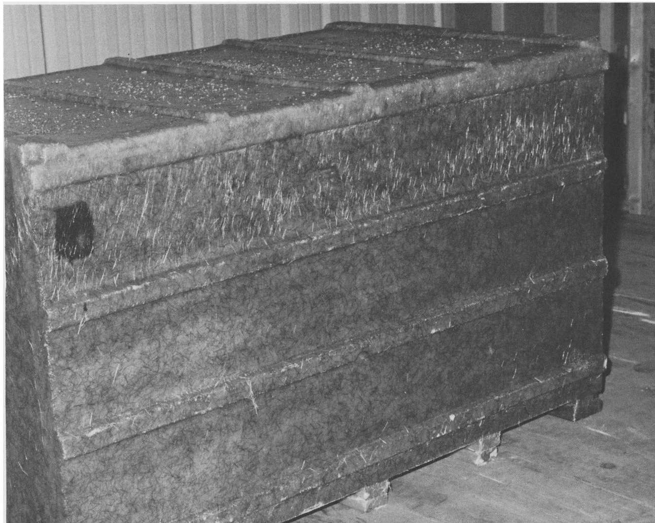
Fig. 2. Large items are packaged in \frac{3}{4} -in.-thick plywood boxes coated with \frac{1}{8} in. of fire retardant fiberglass-reinforced polyester to meet USAEC 20-year retrievability requirement.
