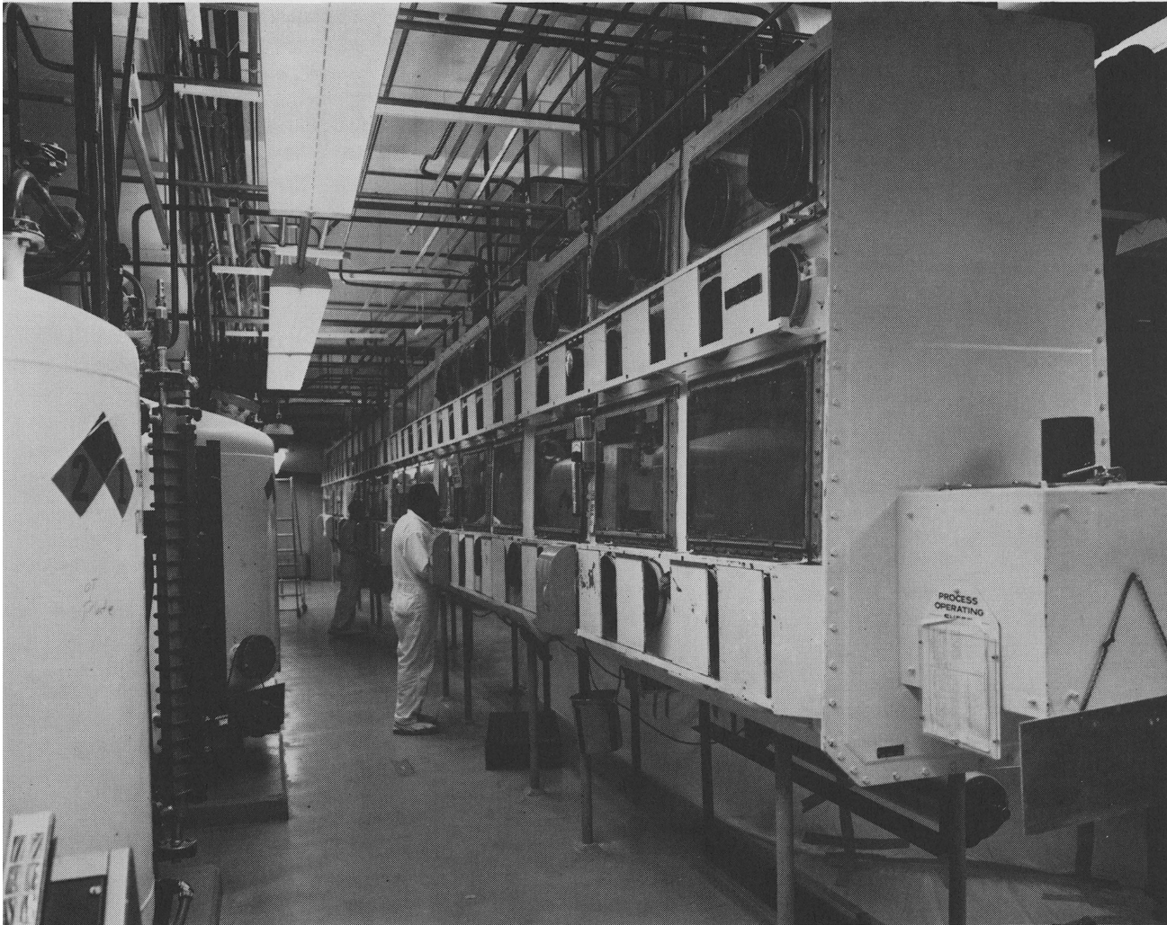
Fig. 1. Rocky Flats handles hundreds of kilograms of plutonium in glove boxes each year.
